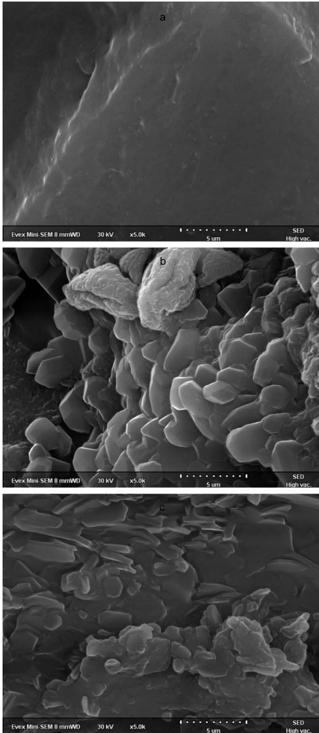
Figure 7. Scanning electron microscopy images of TPU-1 polyurethane specimens: (a) initial specimen without plasticizer, (b) specimen with 30% DPP, and (c) specimen with 30% BTU.
